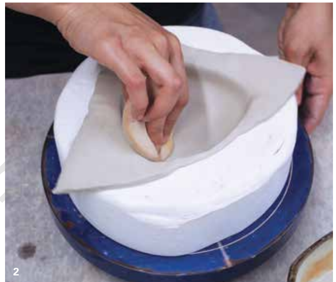
2 Roll out and rib a ½–¾ inch-thick slab. Gently press it into the mold. Use a damp sponge to press into the corners of the mold.
