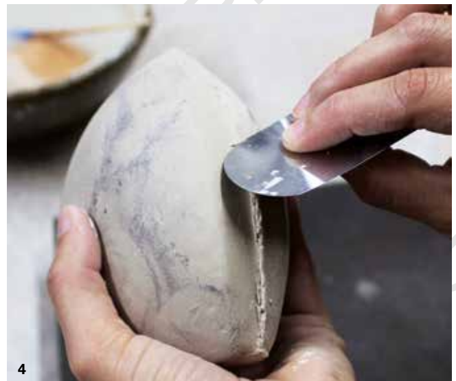
4 Score, slip, and attach the two leather-hard halves and rib the seam to compress the join.
