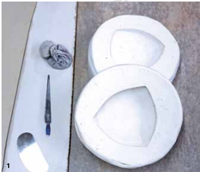
1 Start by powdering the mold using a small piece of tight-knit cloth filled with cornstarch and tied with a rubber band.
