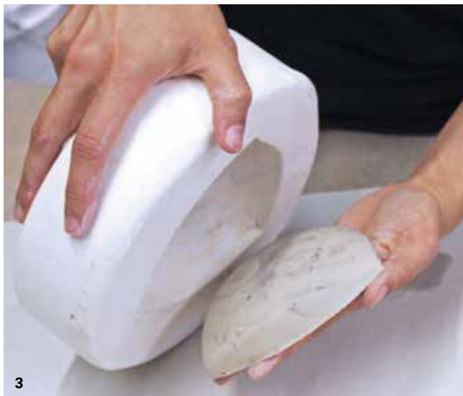
3 Flip the mold over to release the half. Set it aside to firm up to a soft leather-hard state.
